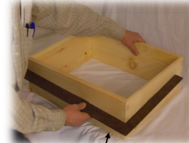
STEP 3: Use your square to check whether the box is square.
