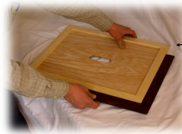
STEP 7: Lay the side of the inner cover with the widest lip up. Nail two nails in each corner— one that goes through the tenon on the end rail, and another that goes through the plywood panel.
