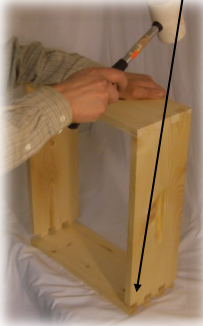
STEP 5: Turn on side and nail with one 6d (8d for greater strength) sinker in each finger in each corner.
