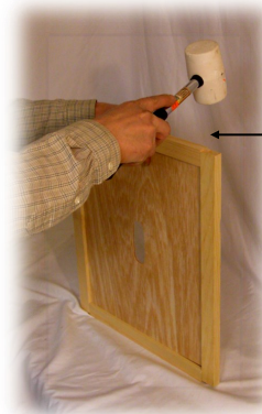
STEP 5: Using your mallet, hammer all four corners to make sure they are even with each other.
