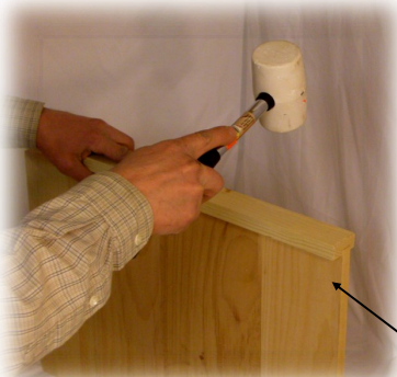
STEP 2: Drive side rails onto tongue and groove panels with a mallet.
