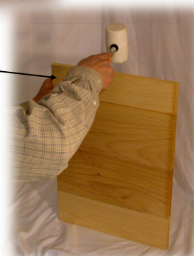
STEP 1: Drive tongue and groove panels together with mallet.
