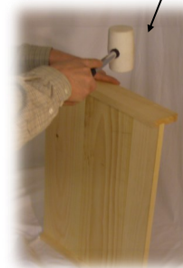
STEP 2: Drive end cleats onto tongue and groove panel with a rubber mallet.
