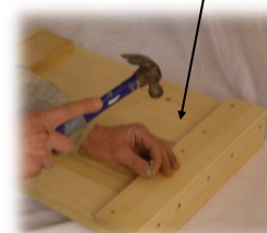
STEP 5: Nail top cleat on, using six 1 1/4" dry-wall nails.
