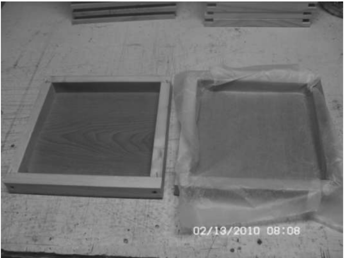
Candy brick molds (These are for making 8x8x1 inch candy bricks but you can make them any size)
